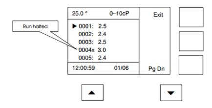
In this case, the temperature, cone, date and time refer to the highlighted line, so as the select arrow is moved down, these values change showing the results recorded for that run. The 'x' on the fourth line indicates that the run was halted prematurely. When limits are enabled, any result outside the pre-set limit values will be shown in reverse video.
