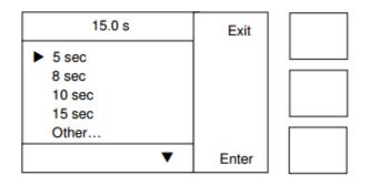
Use the keys to select one of the five options available. The **Other** menu allows any time between 5 and 59 seconds to be set (in 1 second increments). This time should always be at least 15 seconds.
