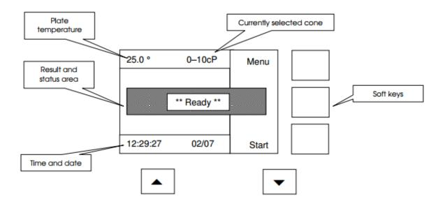
The text displayed next to the three right-hand switches varies from display to display; pressing the switch next to the 'soft-key' will select the function displayed. Using the example above, pressing the top right key will select the instrument menu and the bottom right key will start the instrument.
