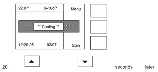
(after allowing the plate temperature to stabilise) the display will change to the one below (assuming the operating handle is up).
