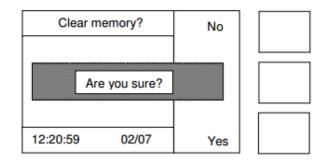
Selecting **Yes** will clear all the stored results and reset the sample id to 0. Selecting **No** will leave the results and Sample id unchanged.
