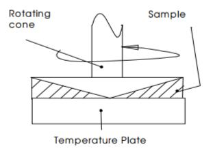
The shear rate (units of s-1) in the liquid under test is dictated by the cone angle ( $\theta$ , units of degrees) and the rotational speed of the cone,  $\omega$  (units of radians.seconds-1) according to the formula: shear rate =  $\frac{\omega}{tan\theta}$  where  $\omega = \frac{2\pi}{60} x rpm$
