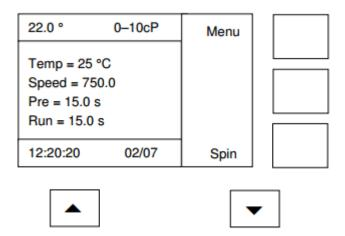
The display will change to one similar to the one shown below a few seconds later. The temperature (top left of the LCD) will flash on and off until the plate reaches the set temperature within its ready band (default  $\pm 0.1$  °C). The instrument will be usable once the temperature has fallen within the ready band.
