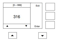
The up and down keys are used to select a new value. The **Enter** key is used to set the new value. The **Exit** key is used to return to normal operation without altering the current value.
