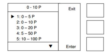
Use the keys to select one of the five cones listed here as the current fitted cone.
