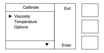
Choose either viscosity (torque measurement) or plate temperature calibration. The options section allows the calibration time to be altered from the default 20 seconds value.
