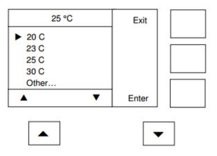
Each line can be selected using the up and down keys. Pressing the down key four times will highlight **Other**. Pressing the Enter key will cause the following screen to appear.
