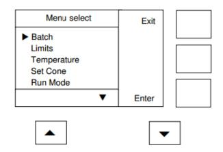
Pressing the down key moves the select arrow down by one line and the screen below will be displayed. The up arrow prompt will appear on the bottom line, showing that the up arrow key is available to move the select arrow back up. Thus the up and down keys are used to move up and down through the menu system. There are more than five menu items and once the bottom of the screen has been reached, the display will continue to scroll down. The full menu items available are:
