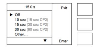
The top line displays the current setting. The values shown are for the CP1 (the values for the CP2 are shown in brackets). Use the keys to select one of the five options available. The **Other** menu allows any time between 1 and 59 seconds for the CP1 (or 1 and 999 seconds for the CP2). The time is set in 1 second increments.
