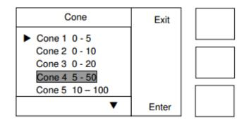
There are 5 possible cones to choose from. Each cone is calibrated separately with 5 oils at a temperature of 25°C for the CP1 (temperature is set automatically during the calibration process). Separate instructions screens follow to lead you through the calibration process - read and follow the instructions on each screen. The whole calibration process can be accepted or rejected at the end. To summarise the process steps:
