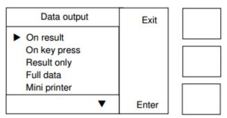
**On result** selecting this causes the data to be automatically output every time a measurement is taken (default)
