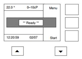
The menu key (top right) is used to access and set various operating parameters - for example, operating temperature. Once the instrument has been set to the required operating conditions, the menu will rarely need accessing.
