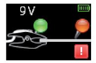
Grounding clamp detected, Coating with defect
