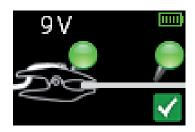
Grounding clamp detected, Coating without defect
