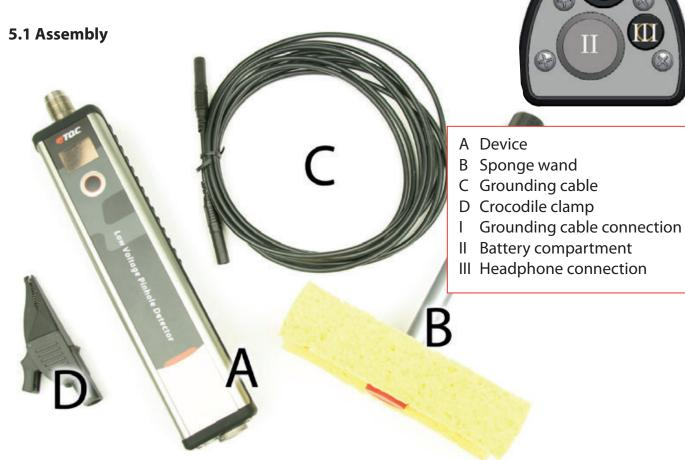
Upon delivery the device (A) and sponge wand (B) will be delivered separately. Before use, they should be connected by means of the screw connection. The 'Advanced' model also has the opportunity to use an extension cable, which offers the possibility to connect the unit to your belt strap. The advanced model comes with different additional accessories that can be used instead of the sponge wand.
